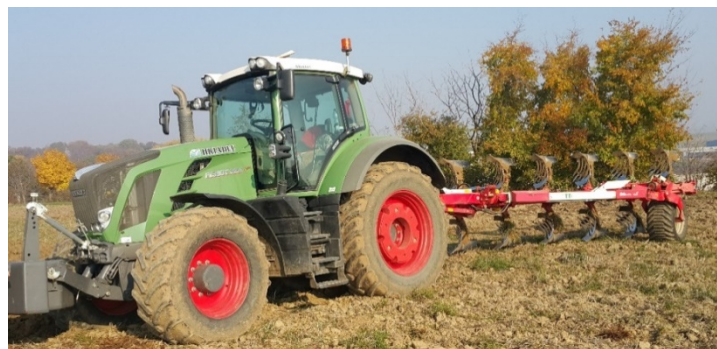
Figure 7. Full mounted 2x7 mouldboard plough with 182kW 4WD tractor
