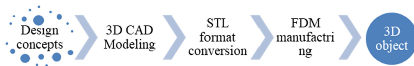
Figure 1. The procedure of FDM printing
