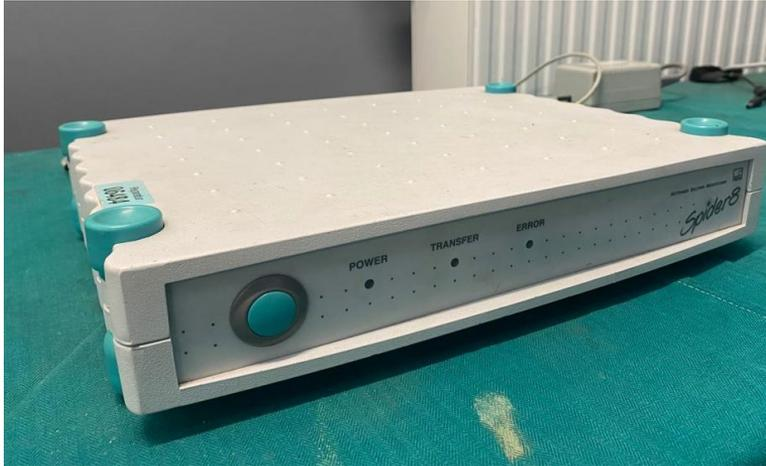
Figure 6. The data logger (Spider 8).
