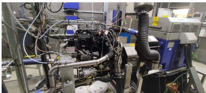
Figure 2. Dynamometer mounted test engine connected to test cell conditioner system
