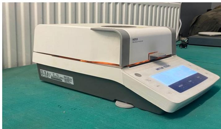
Figure 4. The moisture analyzer instrument (HE53 230 V).
