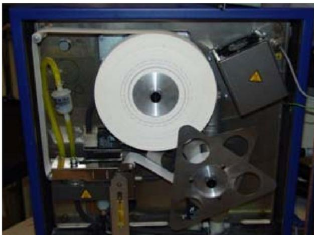
*Figure 6.* Sample paper feeder unit of AVL Smoke measuring equipment
