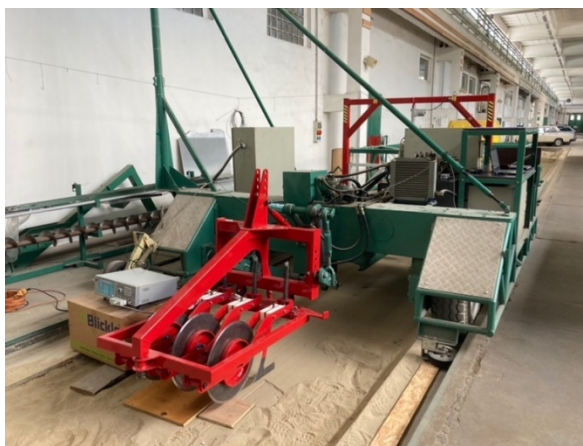
Figure 7. Device carrier, measuring instrument and implement in test position prepared for measurement
