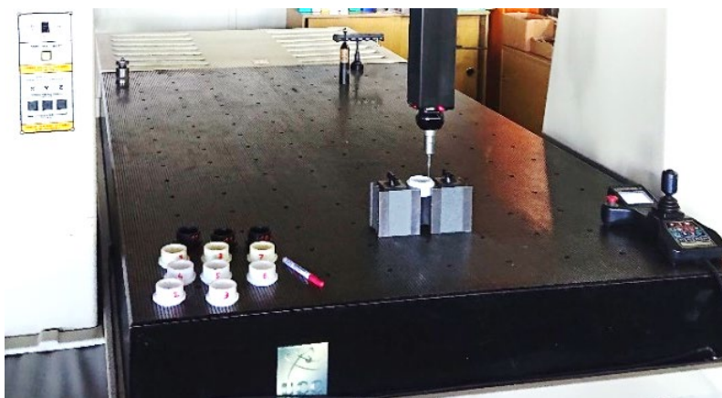
Figure 5. The Gidding&Lewis Cordax RS150 DCC calibrated CNC coordinate measuring machine with Renishaw probe
