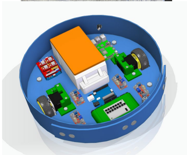
Figure 6. Assembled representation of the robot vacuum cleaner (without top element).
