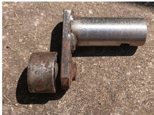
Figure 4. Rotating pin in plain bearings before use
