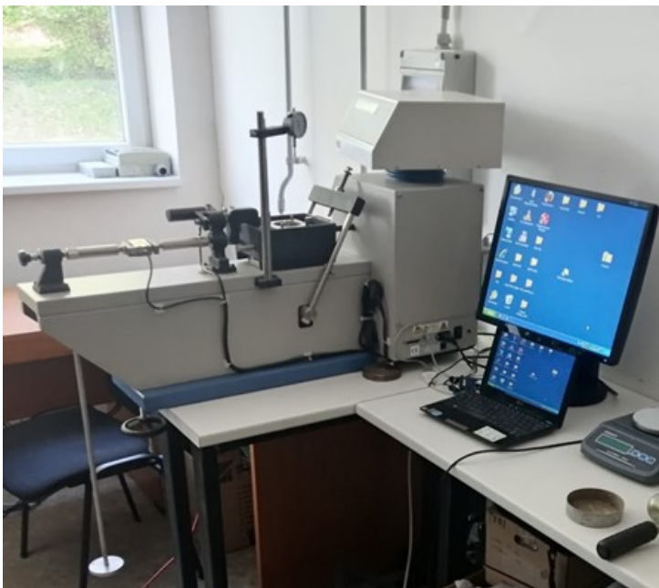
Figure 2. Direct shear test machine (ELE 26-2112/01)
