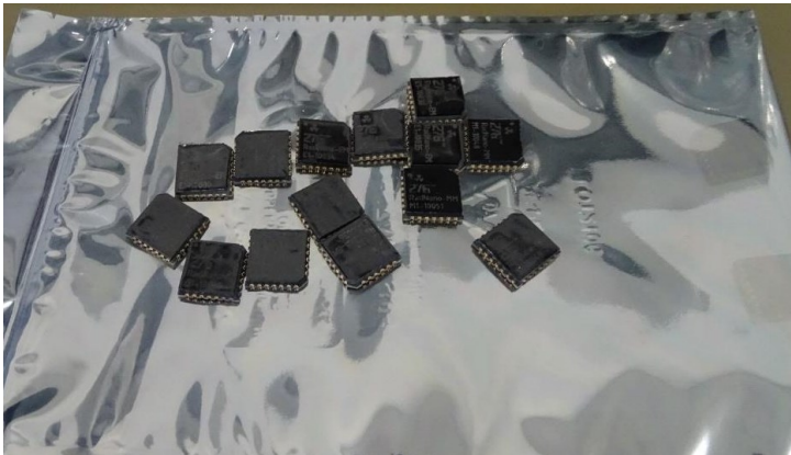
Figure 11. RadNano samples after the test procedure, no visible changes occurred on the samples
