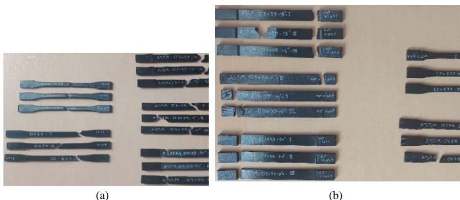
Figure 11. The specimens broken area: (a) flat orientation, (b) on-edge orientation
