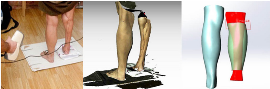
Figure 9. Scanning for preparation of a leg rehabilitation and the printable model (Source: 3dprintingireland.com)
