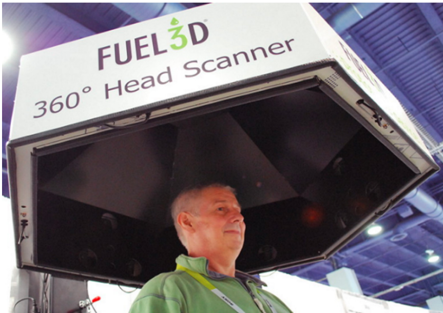
Figure 25. Head scanning using Scanify scanners in a ring, using them simultaneously (source: 3dprint.com)
